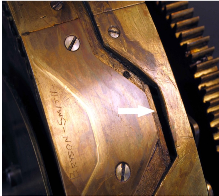
Fig.21. Later zig-zag cam section. Arrow indicating edge of the eighteenth-century cam body and overhang.
