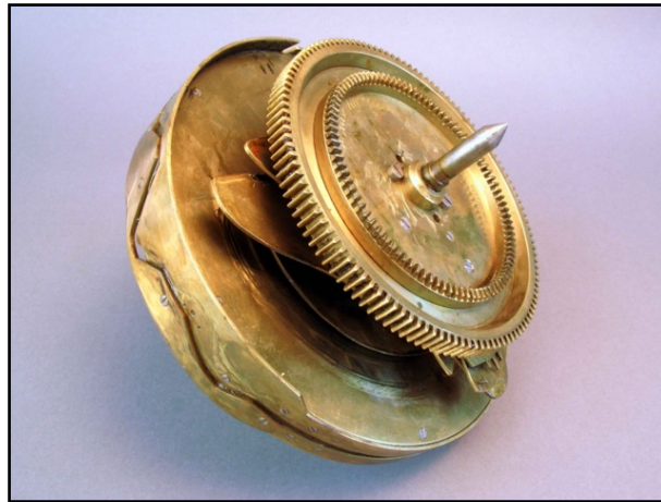
Fig.11. Cat.Ref. x.4653.k.30. The multi-function cam with zig-zag track on the periphery.
