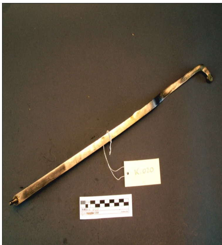
Fig.20. Lower neck operating lever showing signs of wear from rubbing on the edge of the zig-zag track. Cat. Ref. X.4653.k.020
