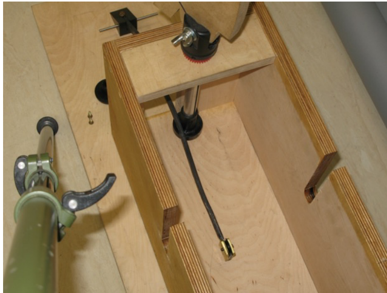
Fig. 46. Test rig lower neck operating lever and associated work in place.
