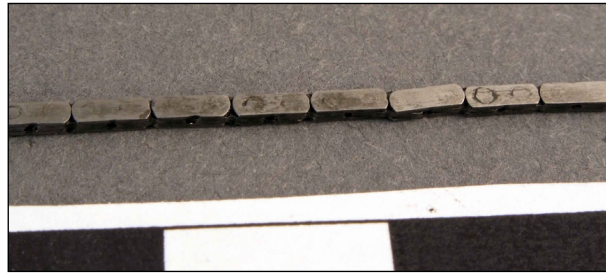
Fig 16. Detail of the neck operating fusee chain (centimetre scale).
