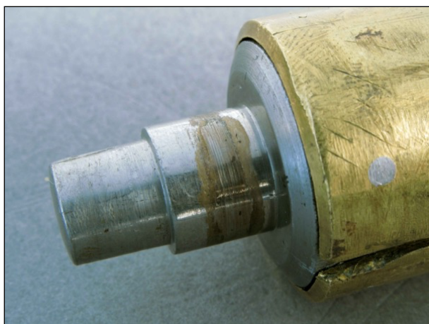
Fig.9. Cat.Ref. x.4653.k.44. Barrel arbor. Wear/damage to bearing surface.
