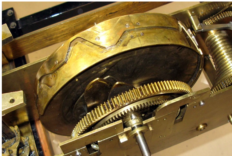
Fig.22. Angular design of the later zig-zag cam elements.
