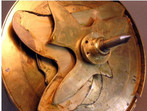
Fig.13. Cat.Ref. x.4653.k.30. Lobed neck operating cams. The cam nearest the cam body operates the lower neck lever.
