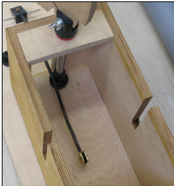
Fig. 33. Test Bed. Plywood box frame detail.
