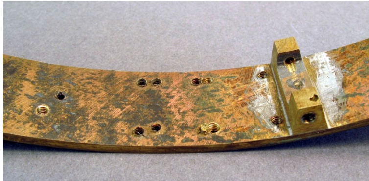
Fig.24. Early smaller diameter holes appear dark and later larger diameter (B.A.) 64 tapped holes appear bright.
