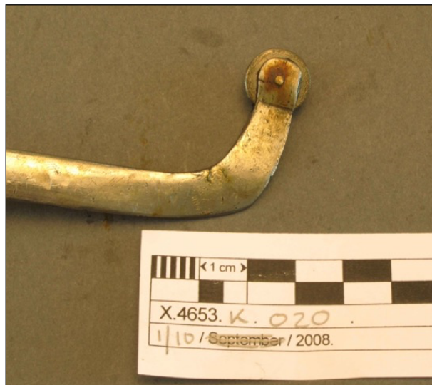
Fig. 17. 18 th Century Lower neck operating lever. Detail of cam roller.
