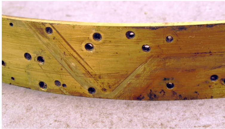
Fig.23. Multiple screw and steady-pin holes; many are now unused.
