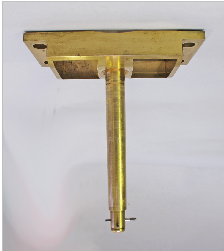
fig. 20 Setting circle spigot and support for the telescope. Enables the instrument to be rotated in the horizontal plane
