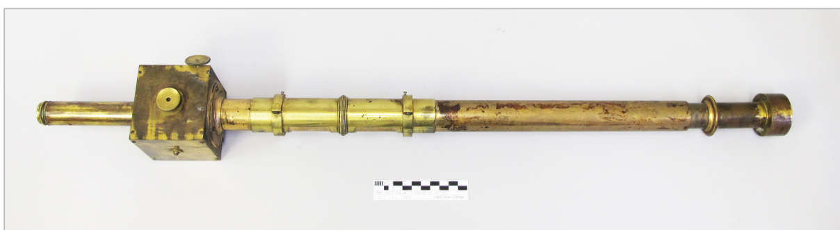
fig. 2 The telescope tube with micrometer box. Overall length approximately 825mm.
