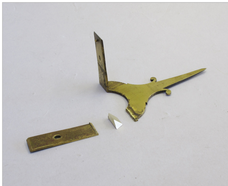
fig. 35 Broken Meridian pointer with a metal reinforcing 'glue block'
