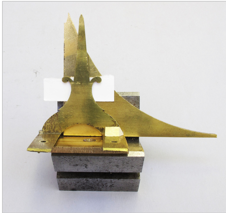
Fig. 36 The Meridian pointer during glueing
