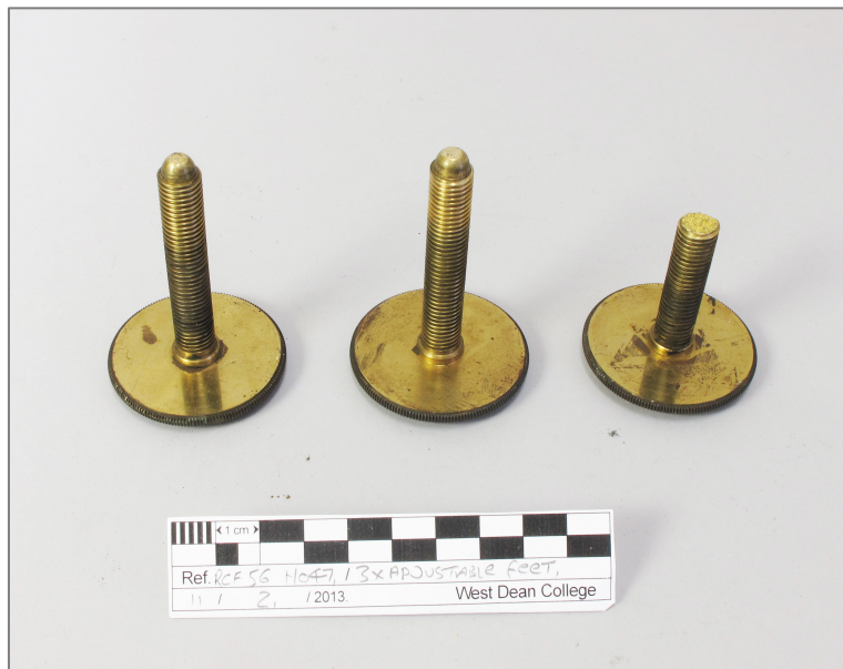
fig. 30 Three tripod levelling screws R. with fractured and lost threaded section.
