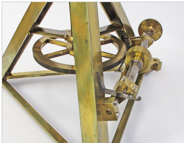
fig. 22 Setting circle worm and pivot blocks screwed to the tripod legs.
