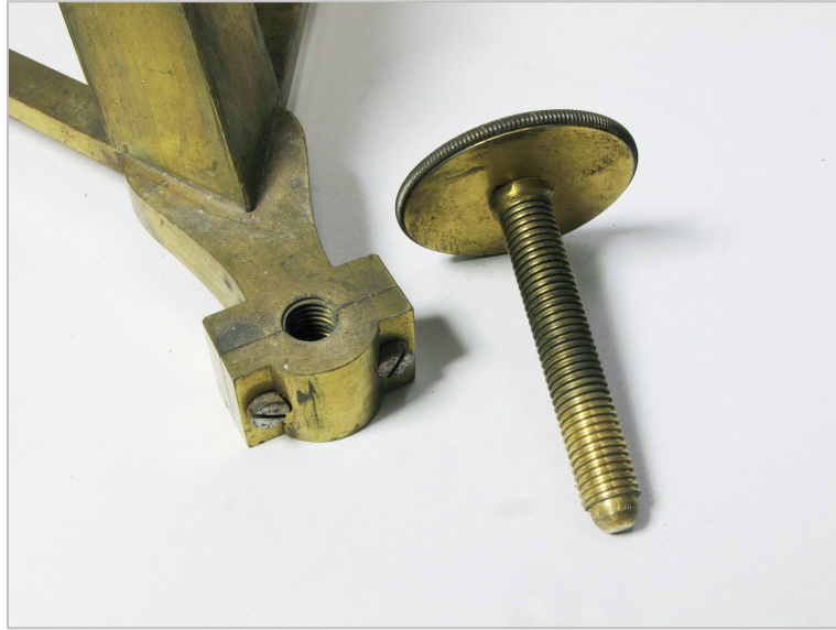
fig. 23 One of the height-adjustable tripod feet and its split clamp
