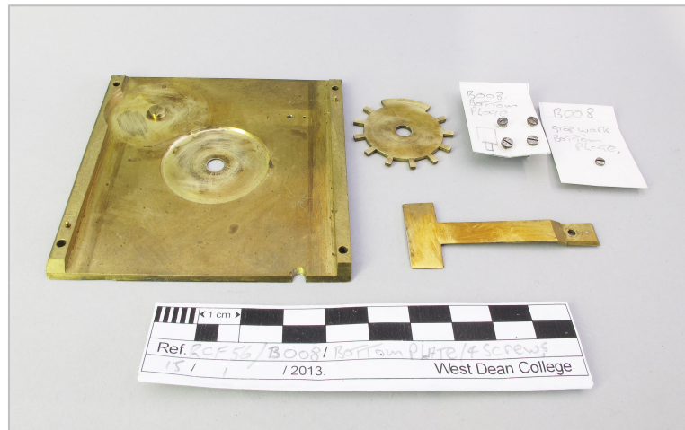
fig.10 Stopwork comprising a wheel with two uncut tooth gaps and a friction spring.
