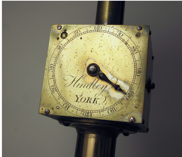
fig. 7 Micrometer box with engraved scale and signature
