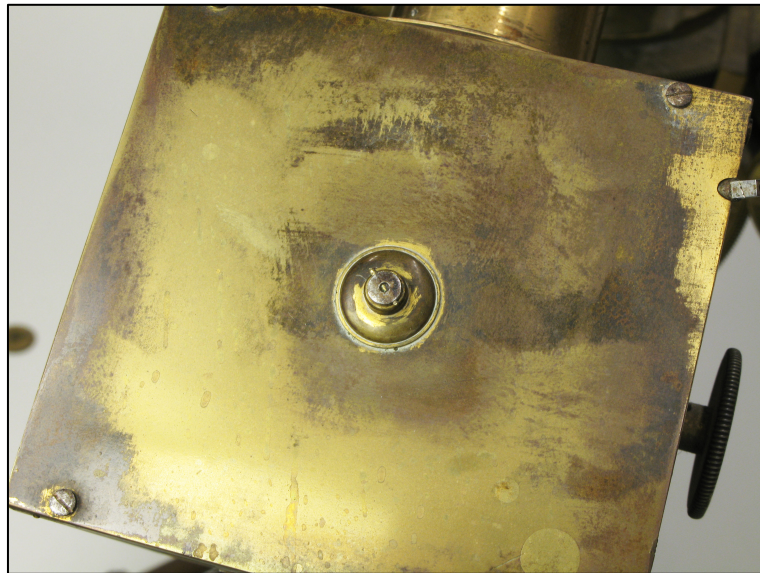
fig. 24 Telescope tube and micrometer box showing losses to the lacquered finish and variegated tarnished brass.
